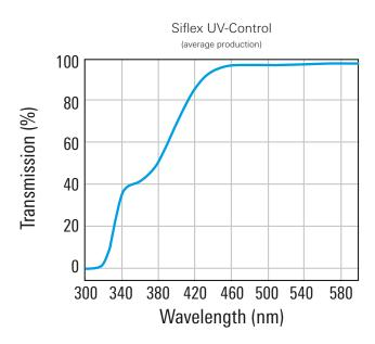
Protective glasses with high energy efficiency an UV absorption are a genuine innovation for shop lighting: **Siflex UV-Control**.
