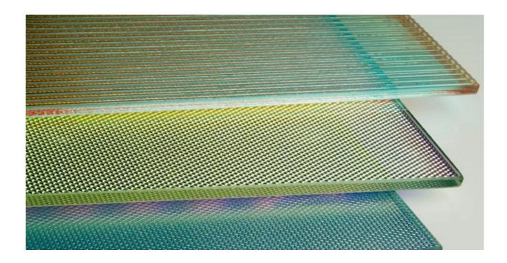
Glasses with specific surface structures e.g. lines, prisms, dots etc, are used for deliberately deflecting and scattering light.
