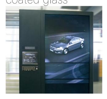
Use as front and protective panels places two fundamental demands on the glass: On the one hand, a high level of transparency is required, e.g. in order to show images or display functions in the best possible manner, while on the other hand, reflections from the surface of the glass must be reduced.
